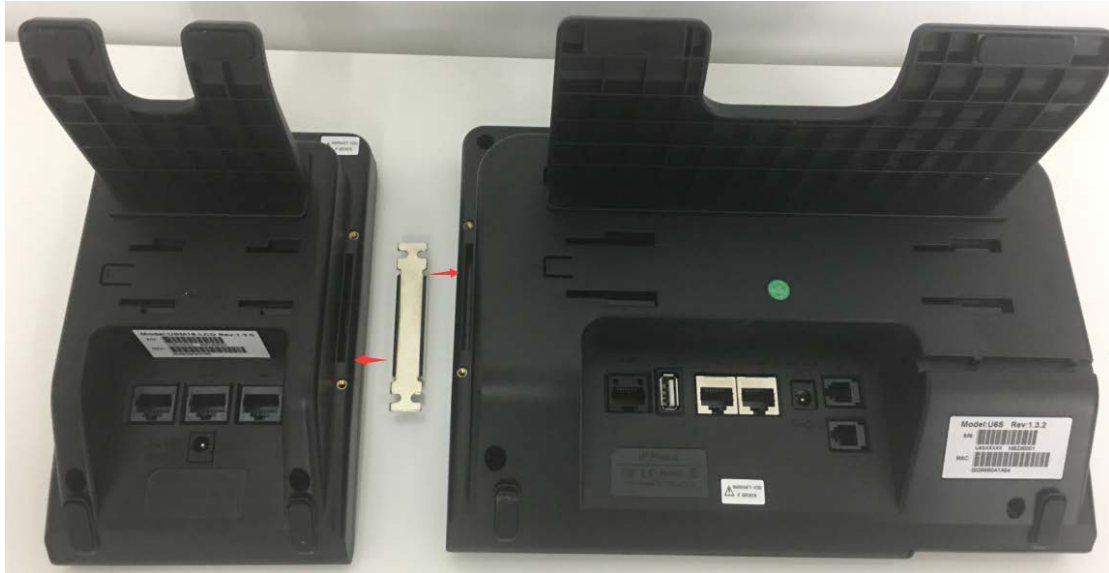
Figure 2.1 ESM18-LCD connect to ES680 IP Phone A
