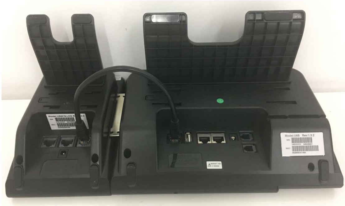
Figure 2.2 ESM18-LCD connect to ES680 IP Phone B
